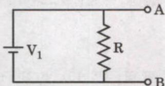
The current through the resistance R is very close to 1 mA and the voltage across point A and B,  $V_{AB} = 1 \text{ V}$ . Now the circuit is changed to :
